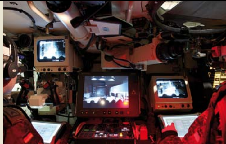
Control units of gunner and commander of AIFV PUMA
